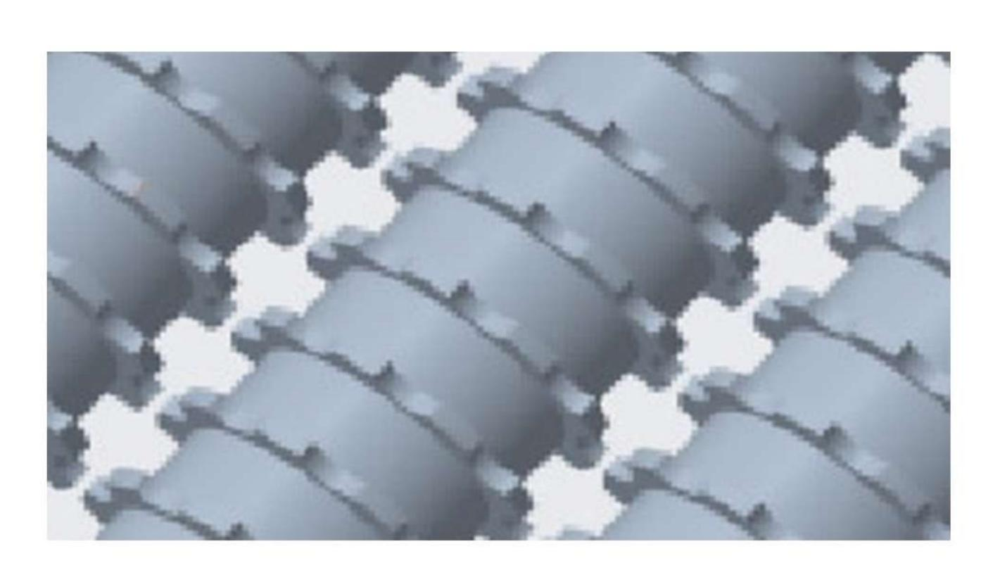
Torx screen disc staggered tooth arrangement
