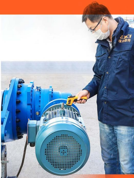
Temperature Rise Testing
