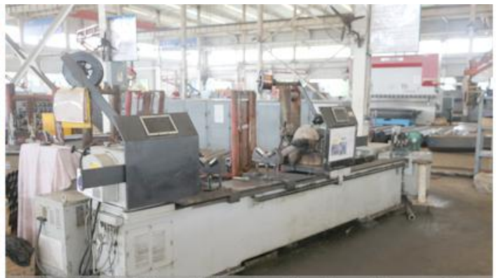
Automatic CO2 Gas-shielded Dual-torch welding machine
