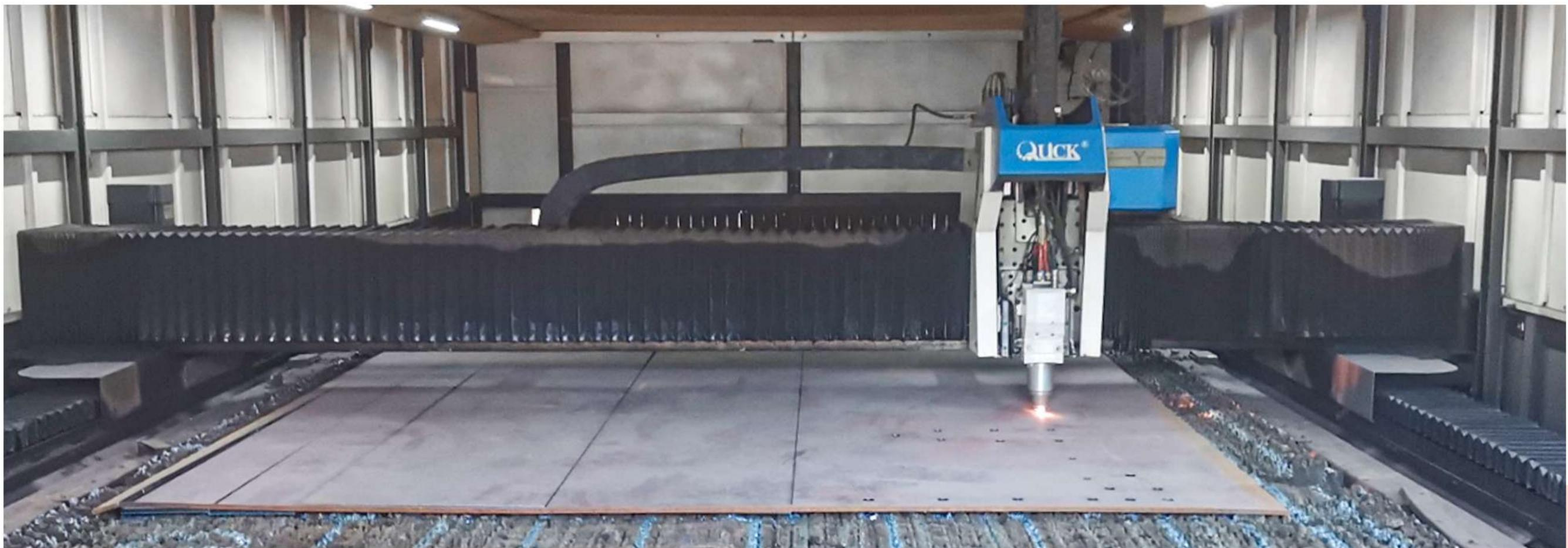
The side plate is made of the whole steel plate in one cut, without splicing. Smooth appearance, beautiful, high precision, manufacturing accuracy ≤±0.03mm, higher than the AS3678–250 standard, to ensure the manufacturing accuracy of equipment. Its flatness error is no more than 1mm per square meter.
