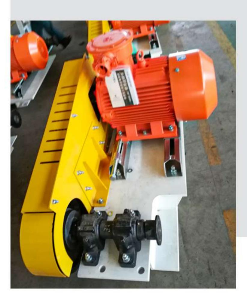
Large and small belt pulley are fixed by expanding sleeve, easy and quick maintenance. The transmission device is equipped with a complete metal protective cover to effectively ensure the personal safety of on-site maintenance personnel.
