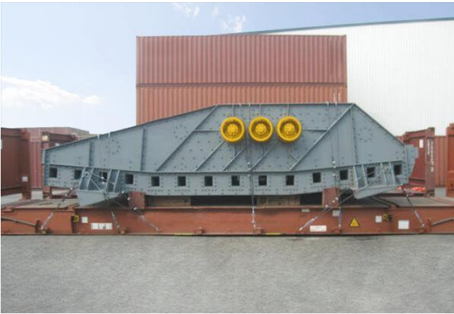
Vibrating Screen Delivery
