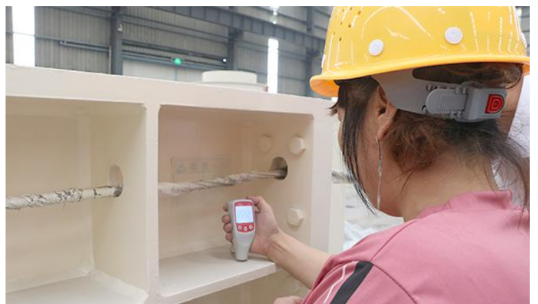
Coating Thickness Check
