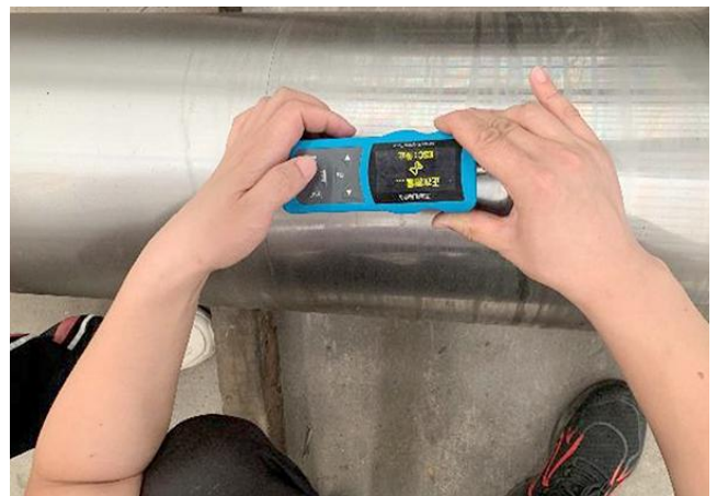
Surface Roughness Test
