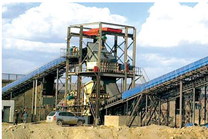
Coal | Neimenggu China | In: 800mm | Out: \leq 250 mm | Capacity: 1,000HTPH
