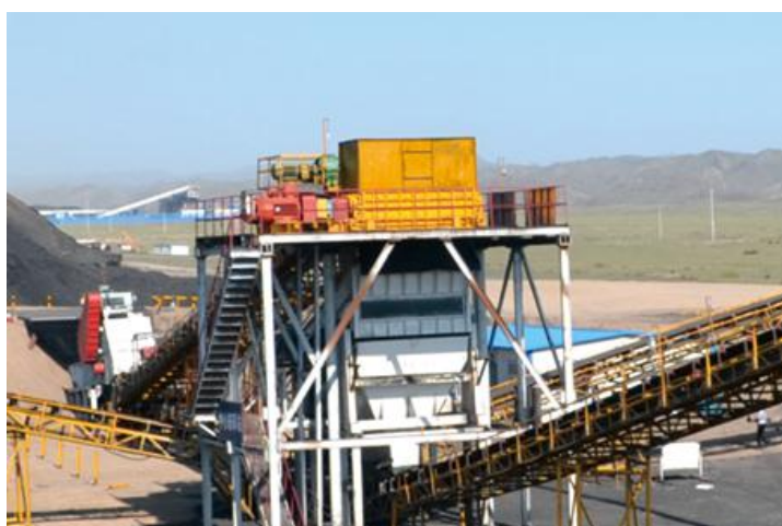
Coal | Shanxi China | In: 700mm | Out: \leq 150 mm | Capacity: 1,300HTPH
