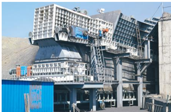
Lump Raw Coal | Sichuan China | In: 600mm | Out: 60-120mm | Capacity: 2,000HTPH
