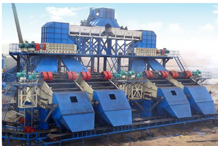
Coal | Bangladesh | In: 350mm | Out: \leq 50-120 mm | Capacity: 5000HTPH
