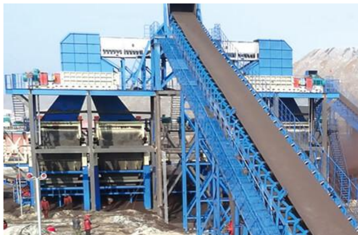
Coal | Guizhou China | In: 800mm | Out: \leq 150 mm | Capacity: 4,000HTPH
