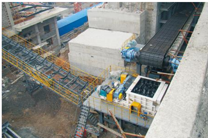
Aggregate | Shandong China | In: 500mm | Out: \leq 300 mm | Capacity: 2,000HTPH
