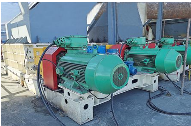
Copper Ore | South Africa | In: \leq 1000 mm | Out: \leq 150 mm | Capacity: 5,500HTPH
