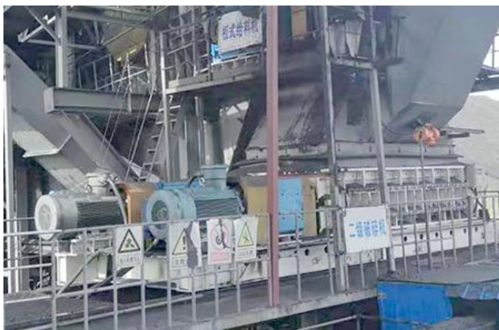
Brown Coal | Canada | In: 1000mm | Out: 200mm | Capacity: 4000HTPH
