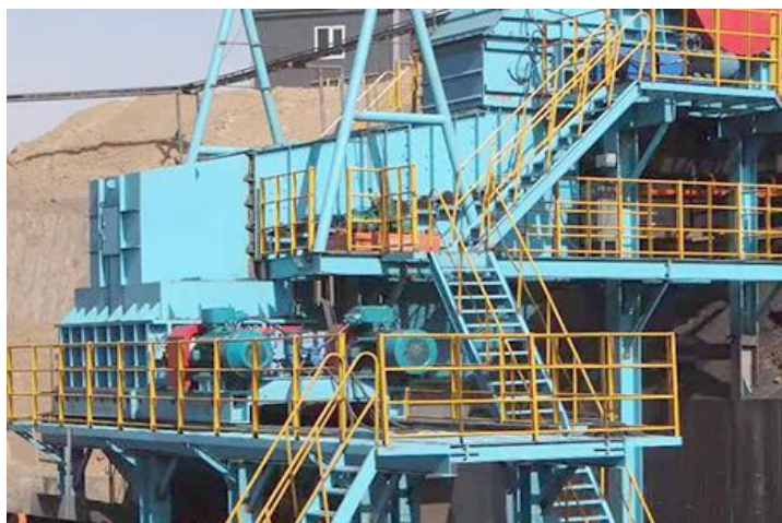
Limestone | Colombia | In: 300mm | Out: \leq 50 mm | Capacity: 3,500HTPH
