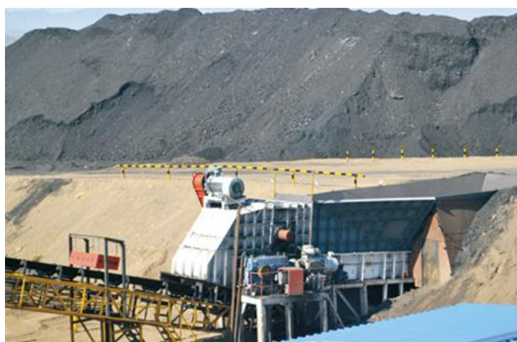
Coal | Guangxi China | In: 600mm | Out: 100-160mm | Capacity: 1,100HTPH
