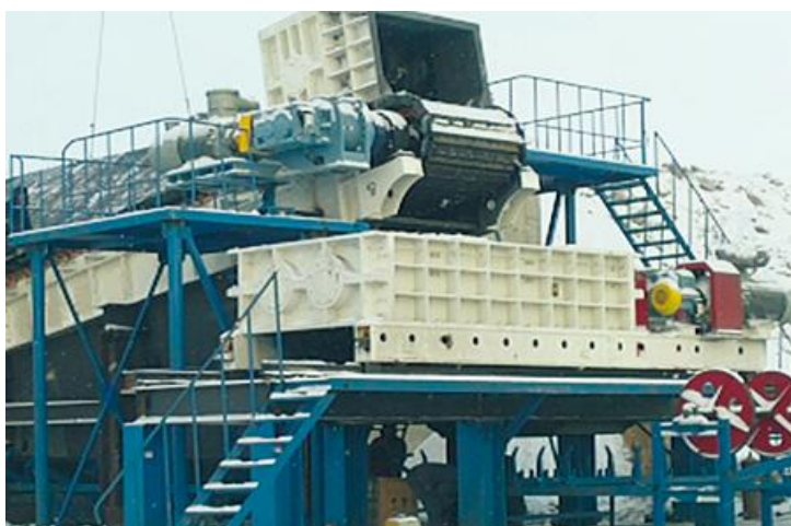
Coal | Xinjiang China | In: \leq 350 mm | Out: \leq 160 mm | Capacity: 3,500HTPH
